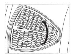
Move the air vent directly to adjust the airflow direction from the horizontal louvres.
